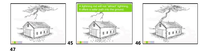
**45:** This sequence of drawings shows how lightning can pass from a storm cloud to a farm building, and the role of lightning protection. Negative charges accumulate at the
